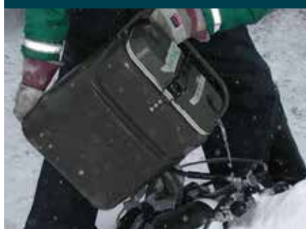
Warm water, from an isolation food container, is used to melt ice on a regulator.
